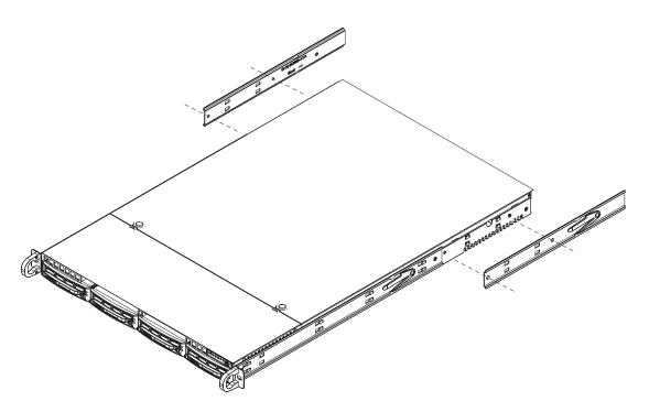
Figure 2-2. Installing the Rack Rails
